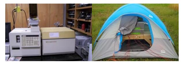
Analysis of soil gas samples can be done using different methods: gas chromatography (GC, left) or laser-based spectroscopy (ie: <u>Picarro CRDS gas analyzer</u>, right).
